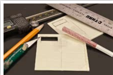
The various tools used to measure, draw and cut the windows from the side panels.
