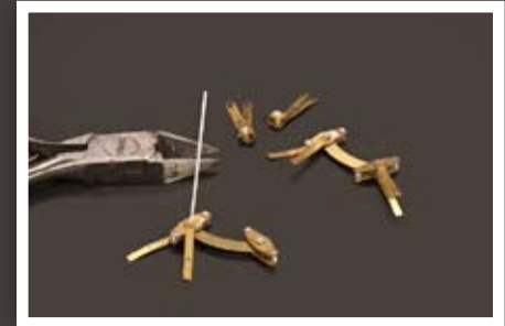
Styrene rod was used as rivets to hold the linkage together.
