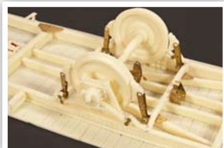
Photo etch details added to the trucks assembly.
