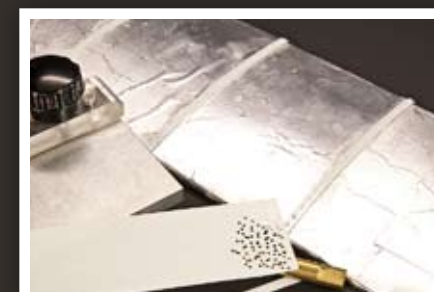
Small rivets punched from plastic stock add the final details to the roof surface.
