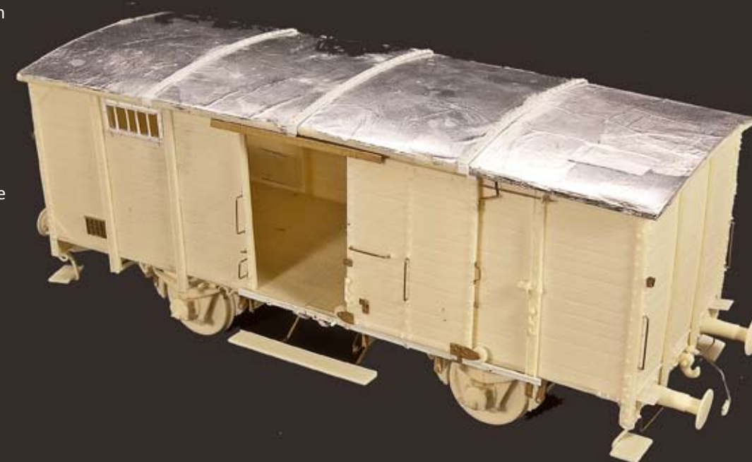
Small rivets punched from plastic stock add the final details to the roof surface.
